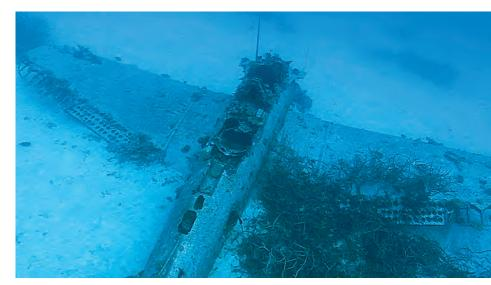
This Dauntless SBD here shows the metal "Swiss cheese" dive brakes on the trailing wing section.
